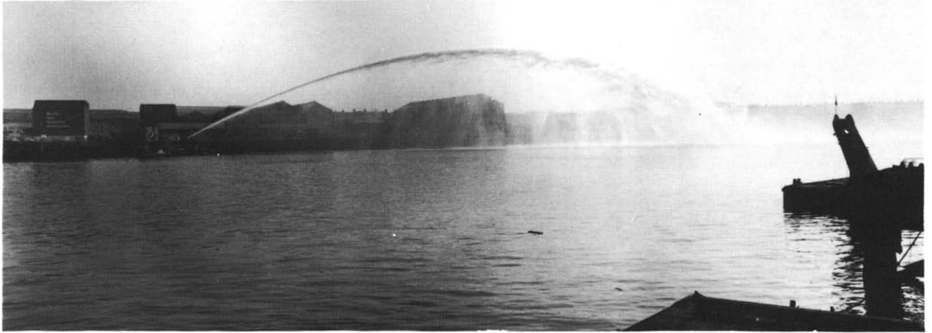
Fig 5 Typical water jet (flowrate 2400 \text{ m}^3/\text{h} , nozzle pressure 12.5 bar)
